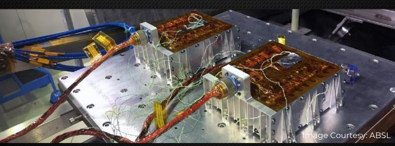
Vibration tests consisted of subjecting each flight battery to vibrations in each orthogonal axis while discharging. The discharge behavior was continuous and smooth through all vibration testing indicating nominal performance.
